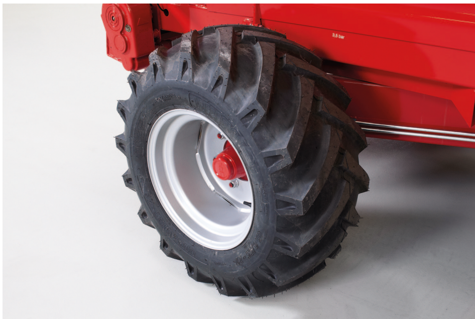
Greater stability is achieved with a low centre of gravity and wide track with tractor profile wheels.
