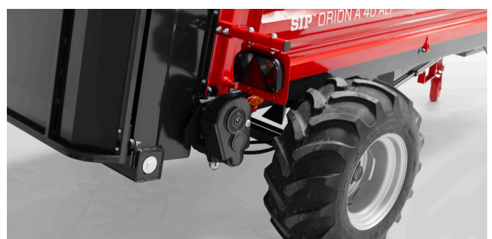
The hydraulic drive of scraper floor and chain conveyor with of 2 chains dim. 10 × 31 mm..
