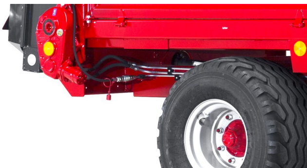
The hydraulic drive of the scraper floor can be continuously adjustable with the lever located on the front of the machine. It can be also moved backward and forward.
