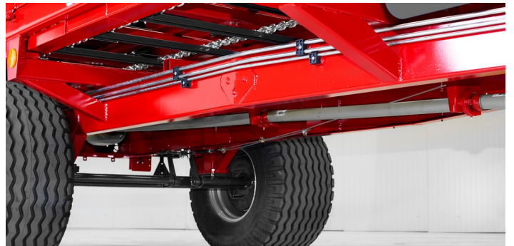
V-shaped chassis with reinforced segments and a stronger axle gives the machine greater stability and load capacity.
