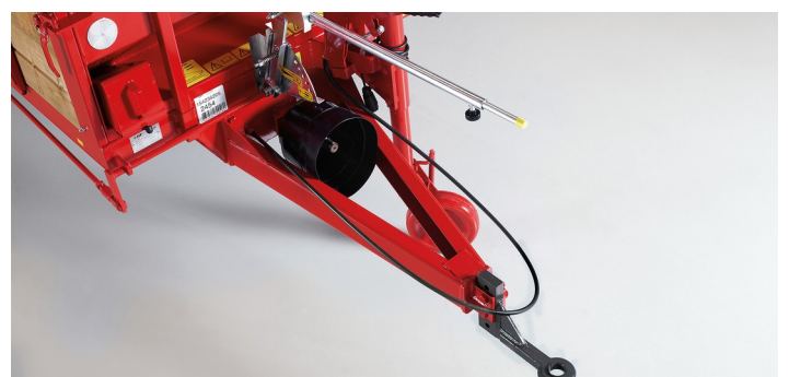
The drawbar linkage is fixed to the lower hitch. The towing eye is adjustable for different heights of tractor hitches.
