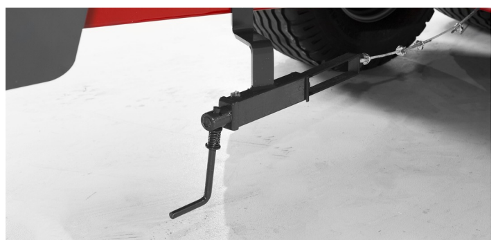
Mechanical brake control via easily accessible lever.
