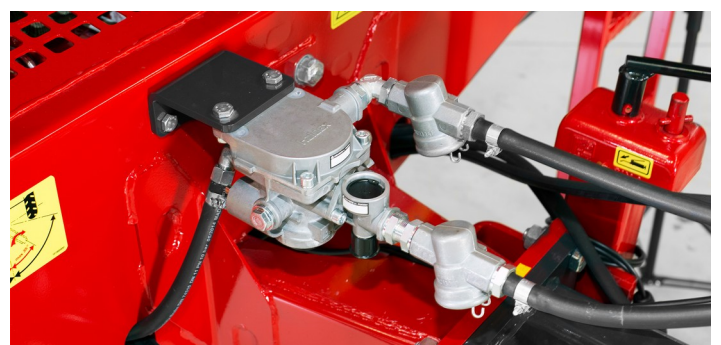
The safe braking with a fully loaded spreader is provided by a double-axle and double-line air brake system with ALB.
