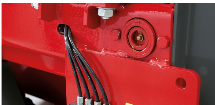
The central lubrication system makes maintenance easier and faster.
