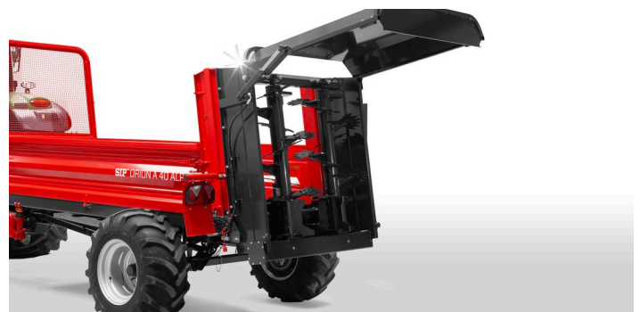
The hydraulic protection of the spreading unit allows easy handling and safe transport.
