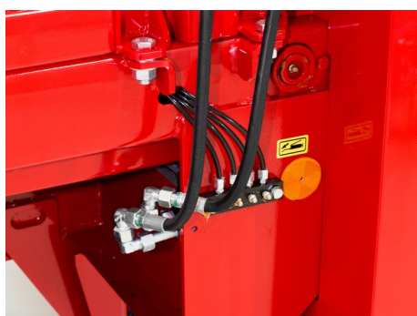
The central lubrication system makes maintenance easier and faster.
