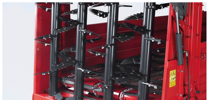
Even spreading up to a width of 10 m is enabled by a spreading unit with four vertical beaters.
