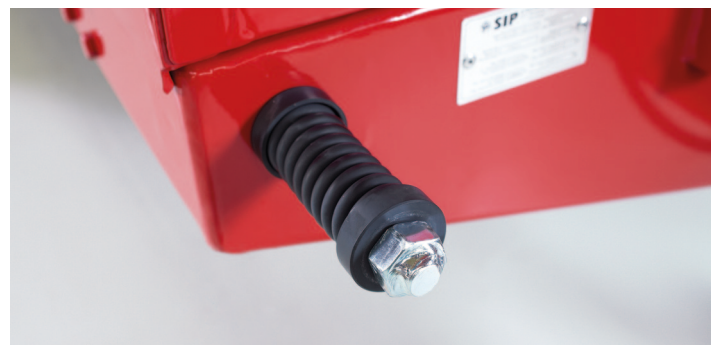
The automatic chain tensioning system (ACT) ensures a constant tension of the scraper floor chains, regardless of the amount of material. The result is efficient and even spreading of the manure.
